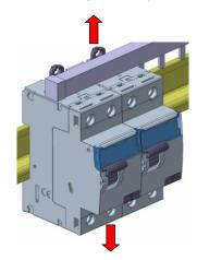
Put the latch clips in the unlocking position
