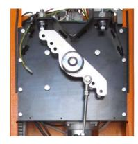
**Balancing springs** - highly robust, guaranteed for up to **3.000.000** manoeuvres for M-Bar and L-Bar models.
