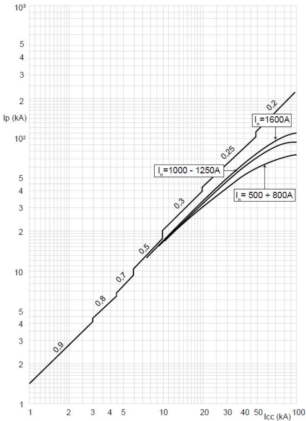
$I_{cu} = 36-50-70-100 \text{ kA}$   $I_{max} = 1600A$  3-4 P  $U_e = 415Vac$
