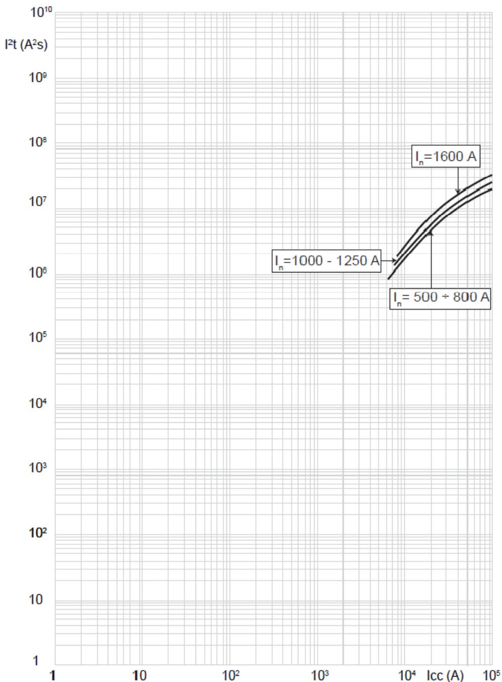
$I_{cu} = 36-50-70-100 \text{ kA}$   $I_{max} = 1600 \text{ A}$  3-4 P  $U_e = 415 \text{ Vac}$
