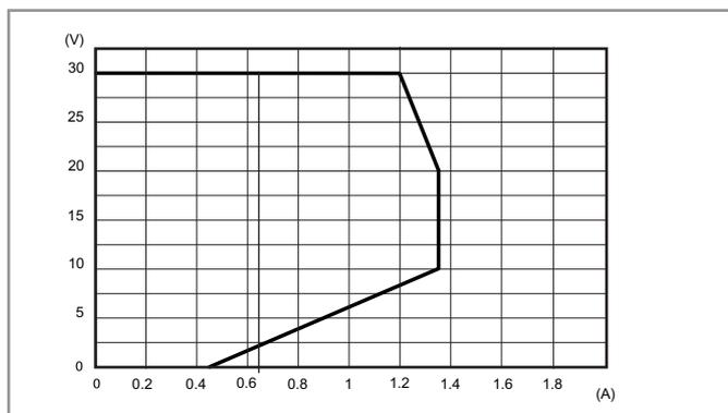
Diagramme de surcharge, conforme KNX
