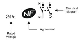
. The terminals upstream and downstream of the neutral pole are marked with an "N" moulded close to the screw heads.
